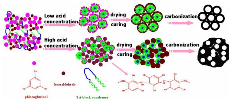
FIGURE 1.11: A possible mechanism of ultra-large pores creation in mesoporous carbons by varying acid concentration [46].
