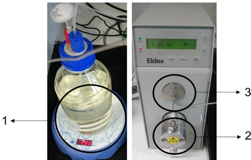
**Figure 6-2:** Continuously stirred reagent vessel (1), plunger pump Eldex 2SMP (2) with pulsation damper (3).
