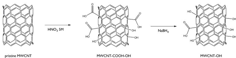
**Figure 4.1.** Acidic oxidation of pristine MWCNTs, followed by reduction using NaBH<sub>4</sub>, yields hydroxyl-functionalized carbon nanotubes (MWCNT-OH)
